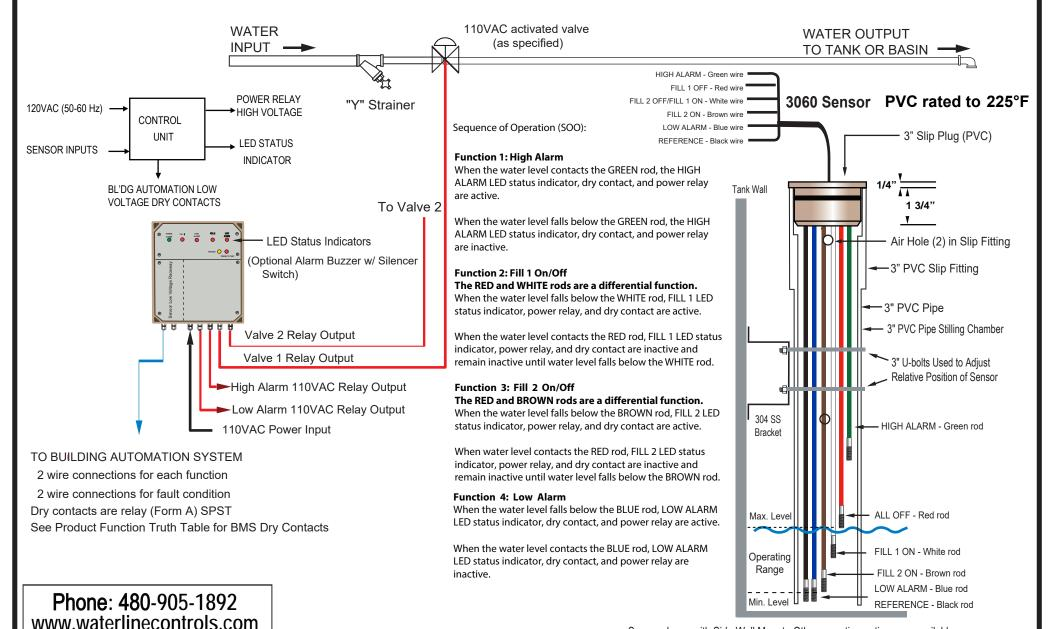
Sensor shown with Side Wall Mount. Other mounting options are available. 3" PVC pipe of length greater than or equal to length of longest rod. Adjust by moving 3" PVC Pipe upward/ downward, then tighten U-bolt.
