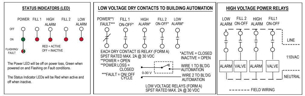
Example of 110VAC devices wired to power relays
