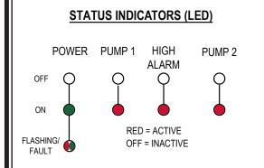
The Power LED will be off on power loss, Green when powered on and Flashing on Fault conditions.
