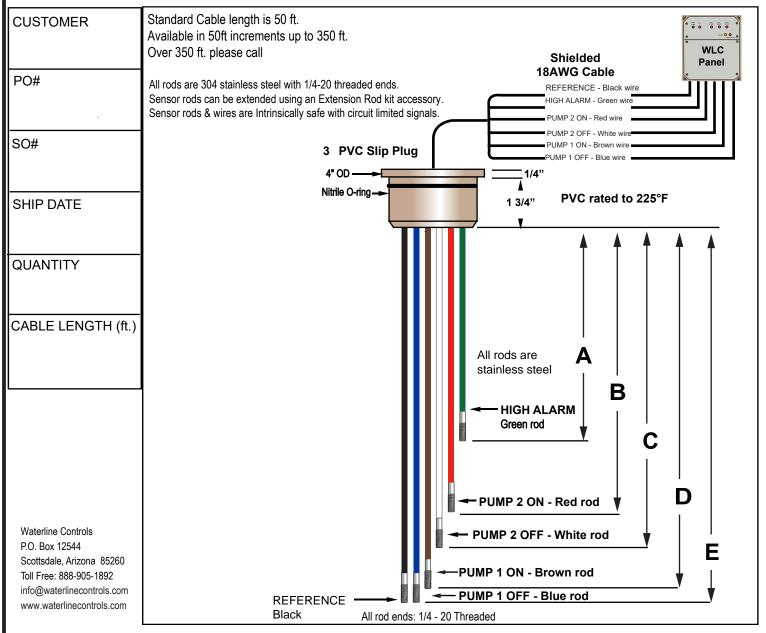
Custom rod length requests should be measured from where the bottom of the sensor cup will be seated after mounting, down to the required function or alarm level(s) in inches. Be sure to take into account any riser pipes or man-way risers
