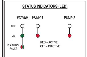
The Power LED will be off on power loss, Green when powered on and Flashing on Fault conditions.
