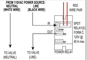
Rated max.: 120 VAC @ 40A All relays are typical All relay terminals are 1/4" male spade
