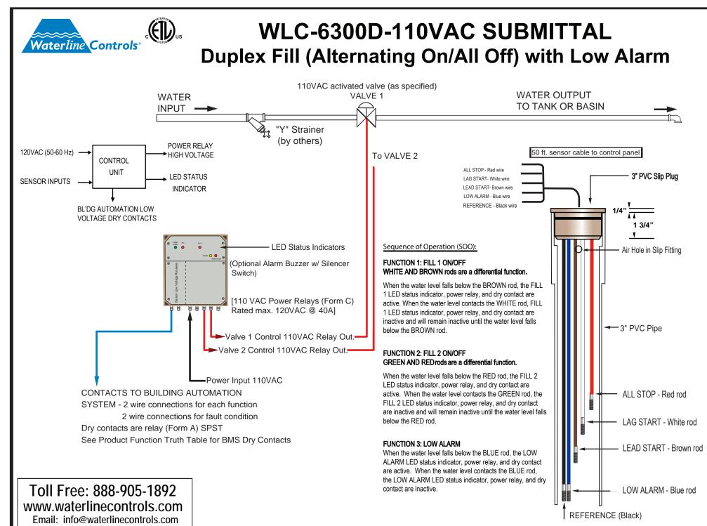
1. 3" PVC pipe of length greater than or equal to length of longest rod 2. Adjust by moving 3" PVC Pipe upward/ downward, then tighten clamp
