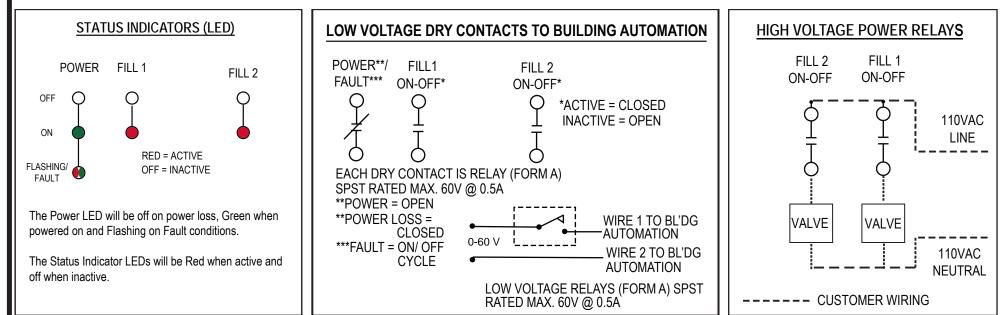
Example of 100VAC devices wired to power relays
