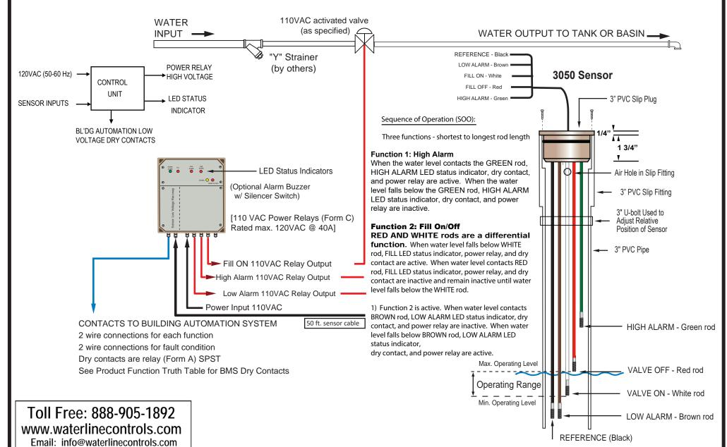
1. 3" PVC pipe of length greater than or equal to length of longest rod 2. Adjust by moving 3" PVC Pipe upward/ downward, then tighten U-bolt WLC-5000-110VAC - 06/29/22
