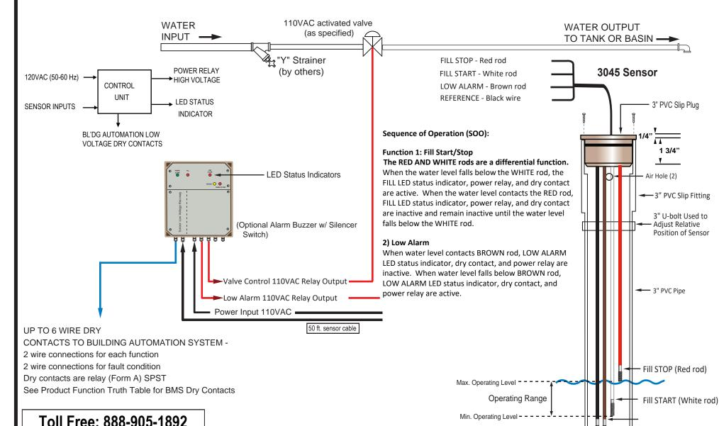
1. 3" PVC pipe of length greater than or equal to length of longest rod
