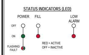
The Power LED will be off on power loss, Green when powered on and Flashing on Fault conditions.
