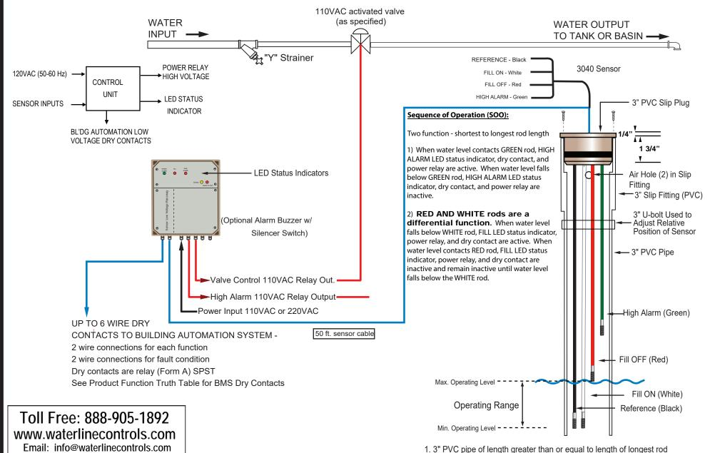
2. Adjust by moving 3" PVC Pipe upward/ downward, then tighten clamp
