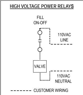
Example of 100VAC device wired to power relay
