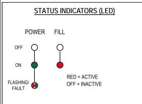
The Power LED will be off on power loss, Green when powered on and Flashing on Fault conditions.
