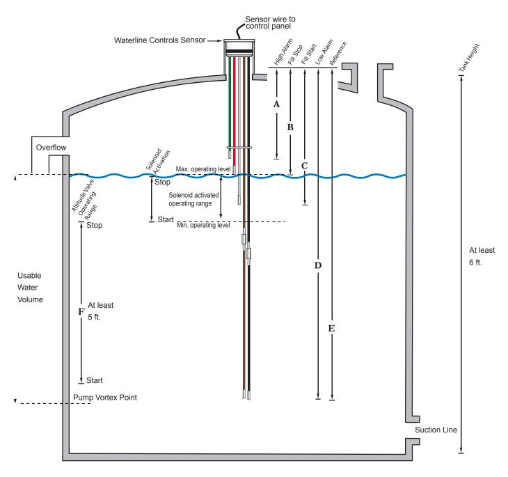
Waterline Controls FPT kits allow the user to maintain NFPA water tank level requirements for the fire protection system. Controling water levels using only an altitude valve results in significant variance in the water level in the tank, insufficient to meet NFPA safety standards. Waterline Controls FPR kits should be used with altitude valves in the fire protection system.
