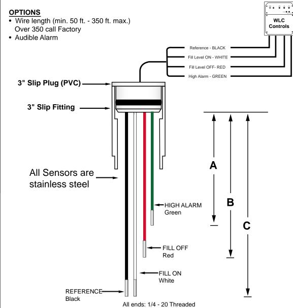
Dimensions should be calculated from the top of the tank or riser down to the required alarm level(s) in inches. Be sure to take into account any riser pipes or manway risers.
