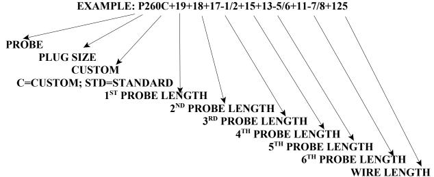
THE EXAMPLE IS FOR A 2" PLUG CUSTOM WITH THE PROBE LENGTHS SHOWN AND 125 FEET OF WIRE. FOR A STANDARD PROBE ONLY THE FIRST 6 CHARACTERS AND THE WIRE LENGTH ARE REQUIRED; ie: P360std+100.
