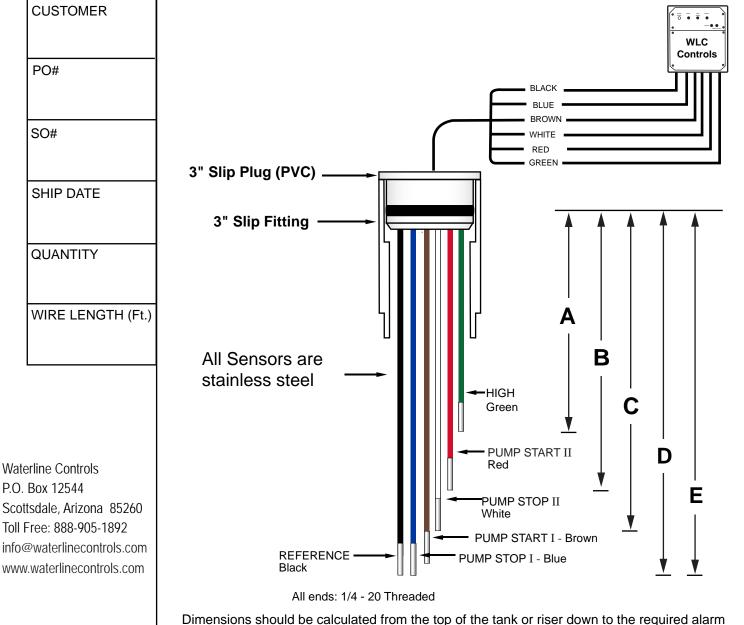
level(s) in inches. Be sure to take into account any riser pipes or manway risers.
