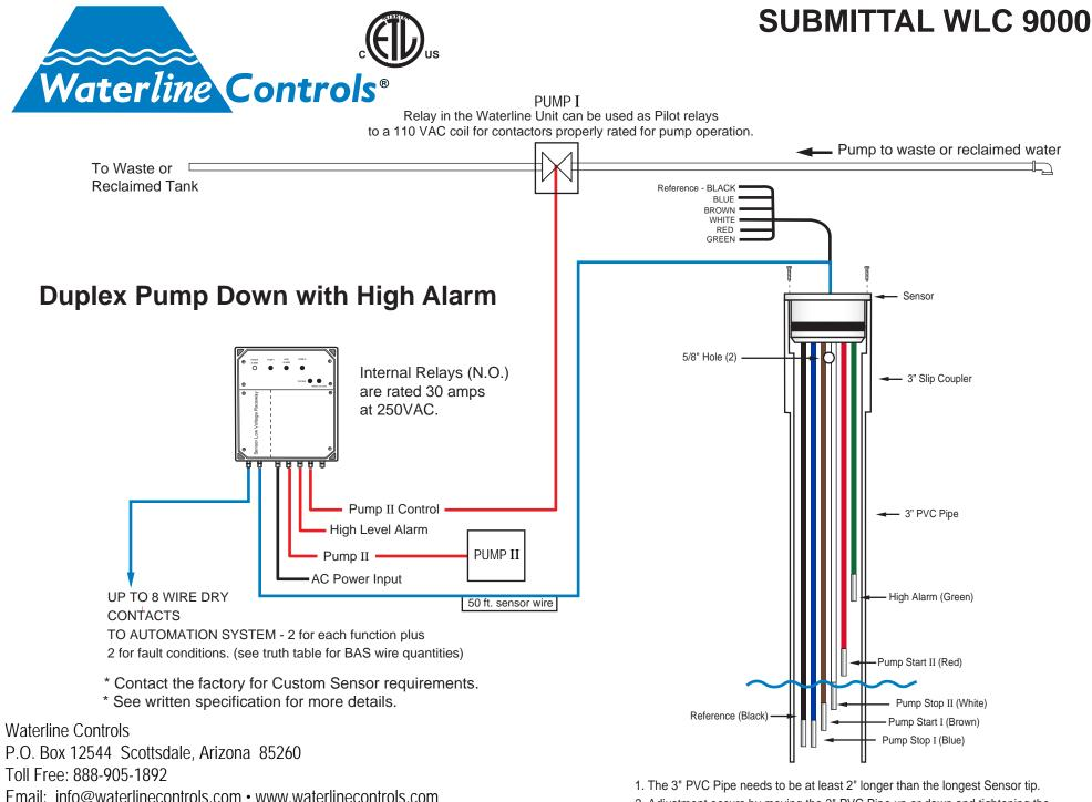
2. Adjustment occurs by moving the 3" PVC Pipe up or down and tightening the clamp so it rests on the Custom Fitting.
