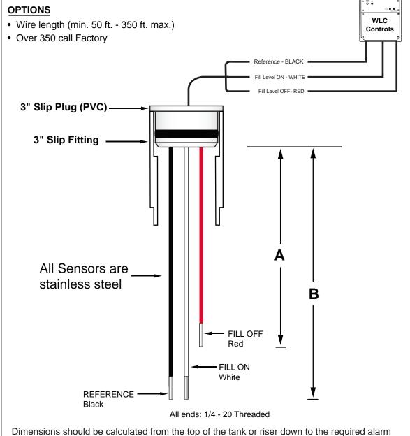
level(s) in inches. Be sure to take into account any riser pipes or manway risers.
